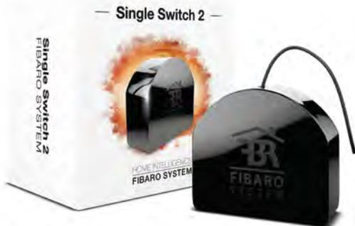
The remotely operated FIBARO Single Switch 2 is designed to turn electrical devices on/off and to measure their power and energy consumption. The compact size of the device makes it the world's smallest of its type and allows for the product to be installed in wall switch boxes or housings to operate an electric device of 2500W of power output. FIBARO Single Switch 2 can be controlled either via Z-Wave network or with a wall switch through a direct connection.
